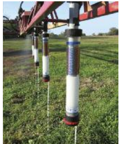
Multiple FlowChecks can be hung on the boom
