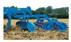
Automatic concave disc adjustment at any working depth
