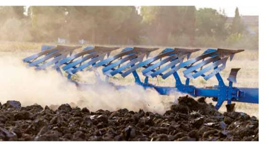
160 x 160 x 10 mm frame strength and a turnover shaft with a 130-mm diameter
