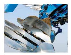
Trash boards for blockage-free work
