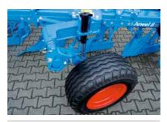
Uni wheel with hydraulic suspension
