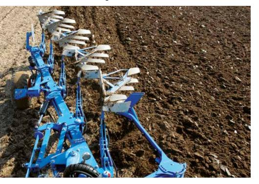
Good ploughing is largely dependent on the working width and the working depth of the individual plough bodies. The LEMKEN Juwel MV can fulfill the agricultural requirements for ploughing in the best possible way.
