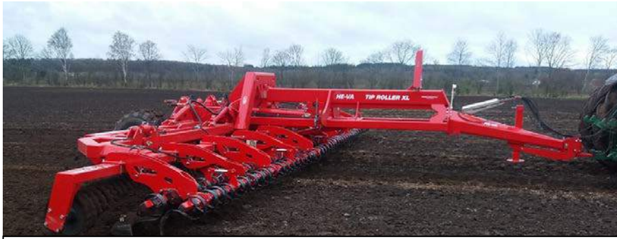
12,30 m Tip-Roller XL with Cambridge rings & 2-row Spring-Board
