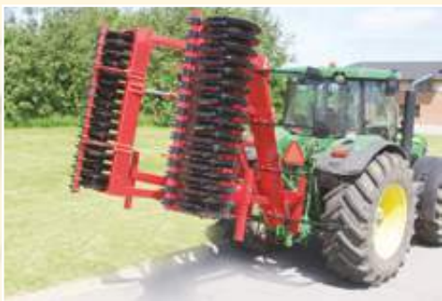
4 m and 5 m models can be folded into a transport width of 2.43 m.
