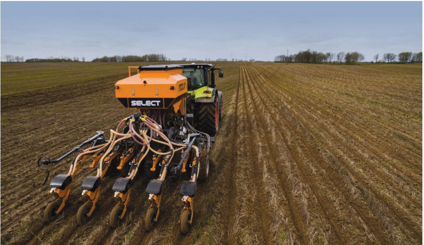
Marking a huge advance in seeding technology, the innovative Mzuri Pro-Til Xzact combines a striptill drill and a precision seeder in just one piece of equipment, meaning that one drill can now seed all types of arable and precision crops – in a single pass.
