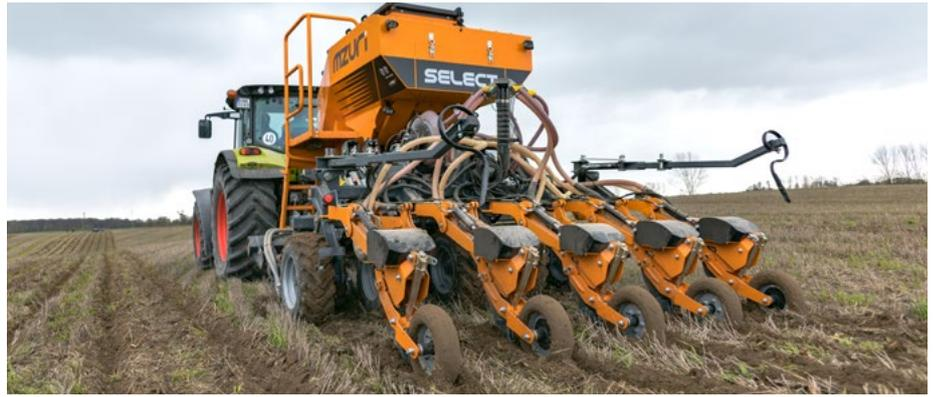
Unlike with conventional precision seeders, the mini hoppers on the Pro-Til Xzact drill are automatically replenished by a bulk fill mechanism on each metering unit directly from the Pro-Til's main tank, thus extending the drilling time and reducing downtime.
