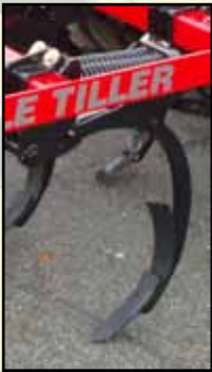
4.00 m trailed Triple-Tiller w/Ø600 mm V-Profile roller and eradicator discs.
