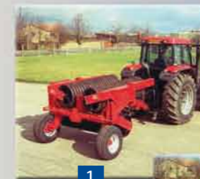
1 Rolls in transport position
