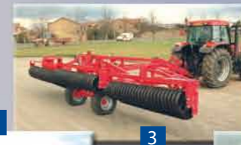
2 3 Swing the wing sections out
